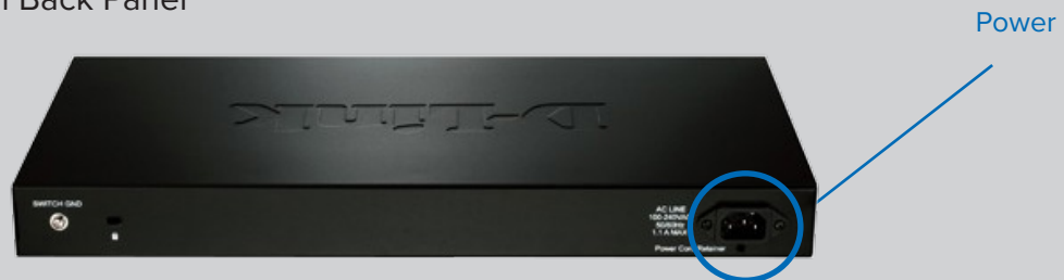
Network Switch Back Panel
