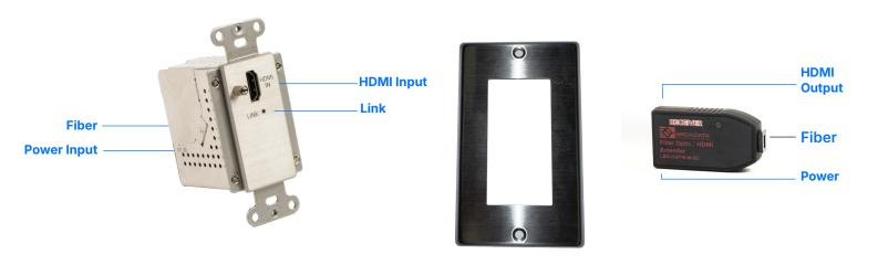
18G/4K HDMI Transmitter 1 Multimode Receiver HDMI Ouput
